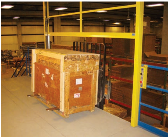
Vertical lift gate
